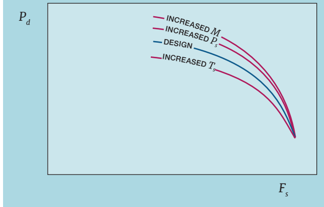
Figure 3: Impact of operating conditions
