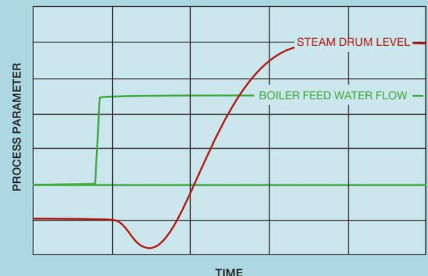
**Figure 4: Three-element level control**
